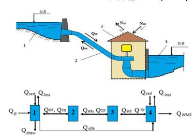
Figure 1: Structural diagram of the PSPP: 1 - upper reservoir; 2 - pressure pipe; 3 - the building of the PSPP; 4 - lower reservoir.
